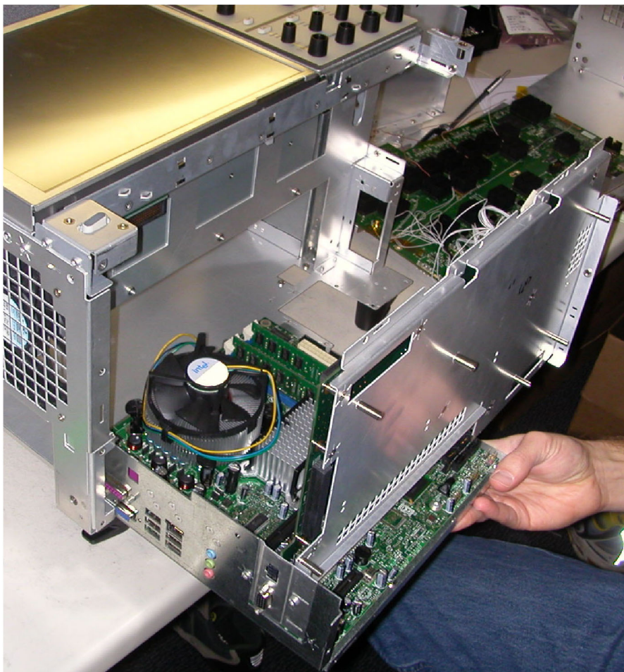
Figure 4-3: Removing the \mu ATX/Power Interface assembly
