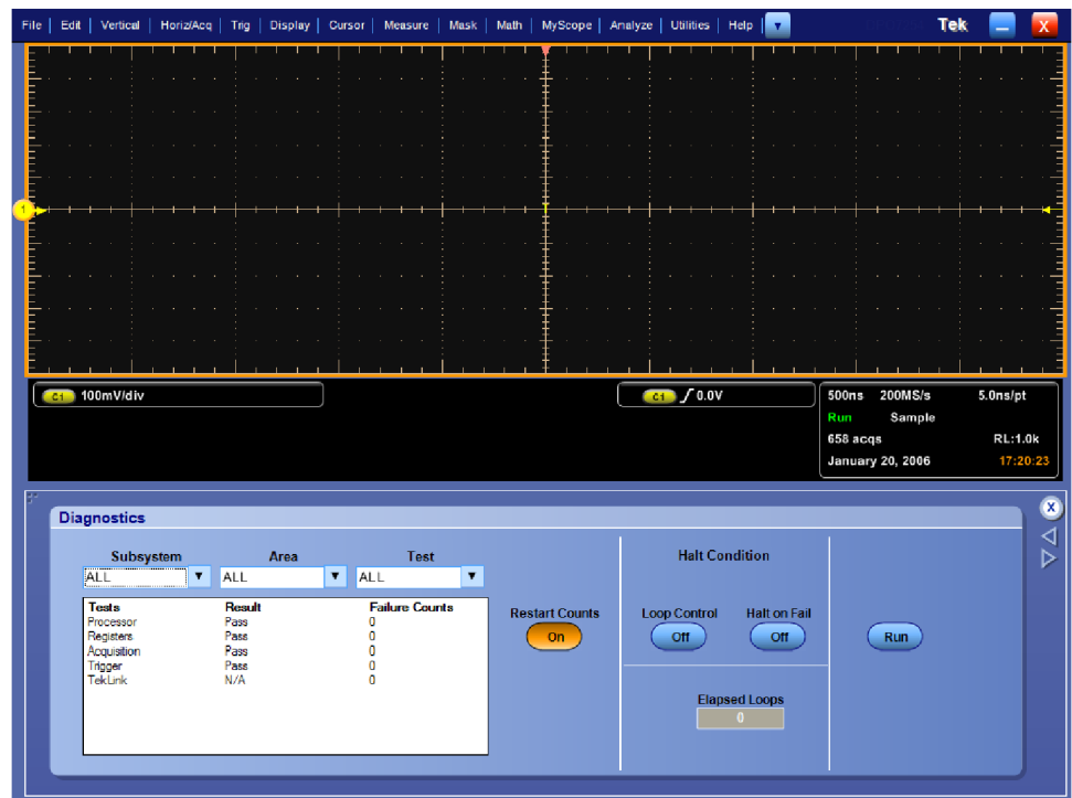
Figure 4-7: Diagnostics control panel
